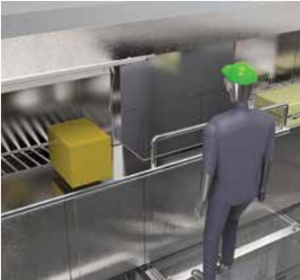
The enclosure of the plant components reduces contamination
