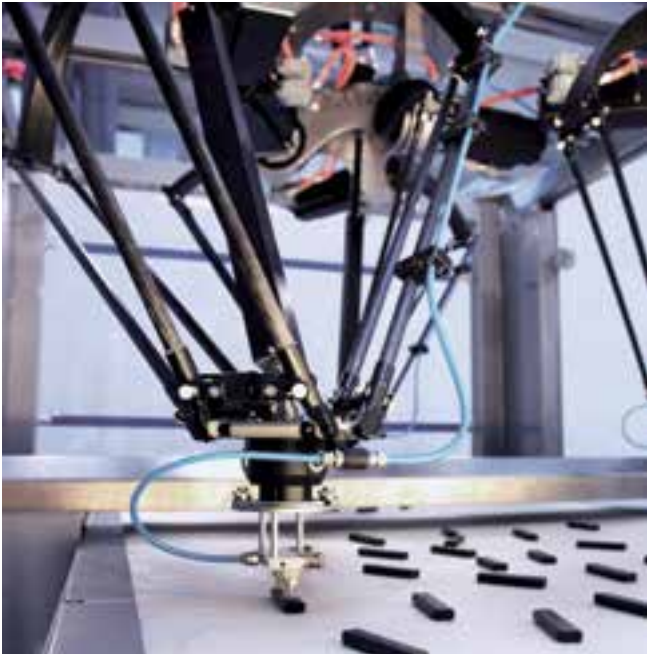
Cama Delta Triaflex robot picking up and depositing chocolate bars
