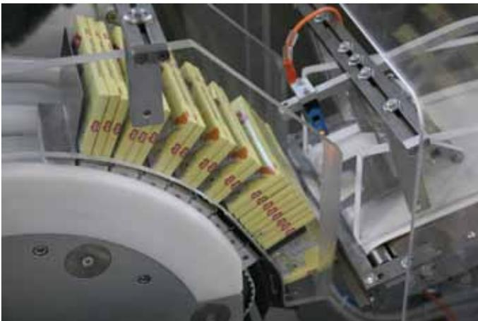
Cama's wrap-around case packer can package up to 360 bars tablets per minute
