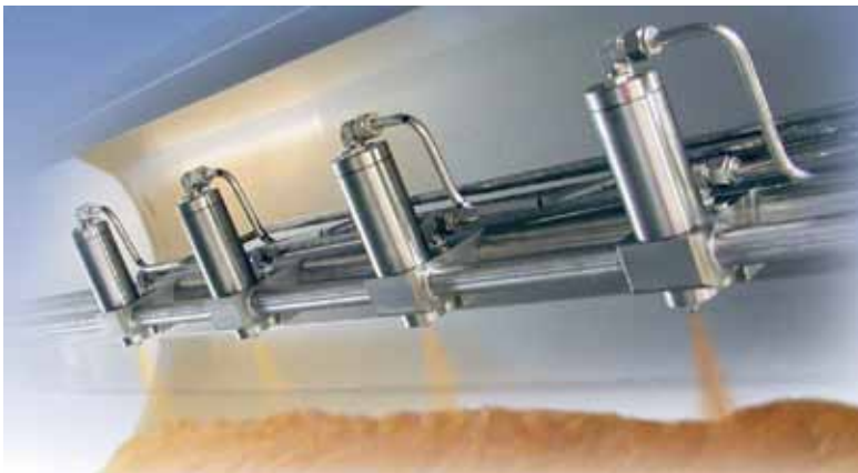
The Spray Dynamic Soft Flight® Coating Drum applies liquid and dry seasonings to extruded, baked, and fried snacks
