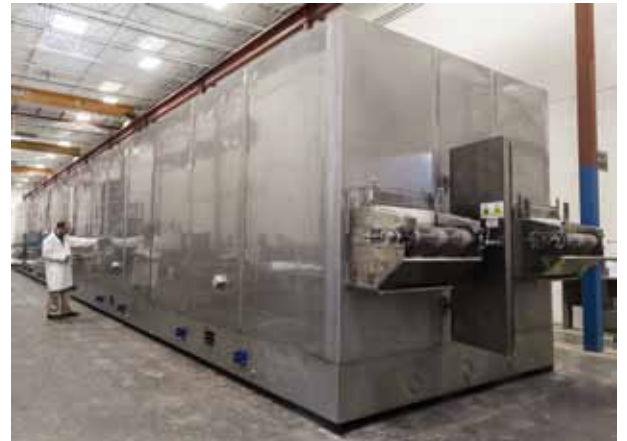
The GEA HVF uses high-velocity air jets to effectively break the insulating boundary layers around the product
