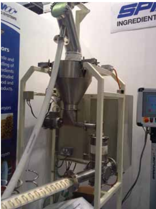
Close up of the Flexible Screw Conveyor exhibit on the Spiroflow stand
