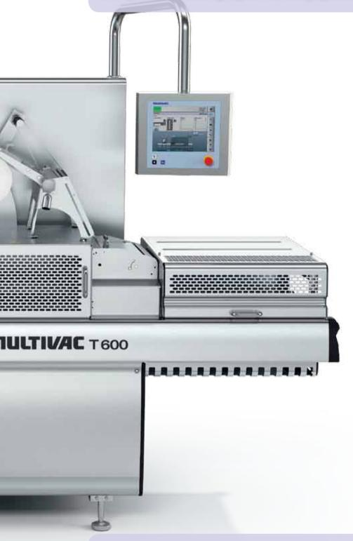
**Multivac**'s T 600 seals up to 40 trays per minute and is directed primarily at small and medium-sized food producers and packers requiring a solution that is compact and capable of being fully integrated in a line. The main application areas of the T 600 lie in the food sector, primarily in meat, sausage and convenience products, but it is also suitable for the packing of seafood/fish and cheese, as well as fruit and vegetables or salad products.
