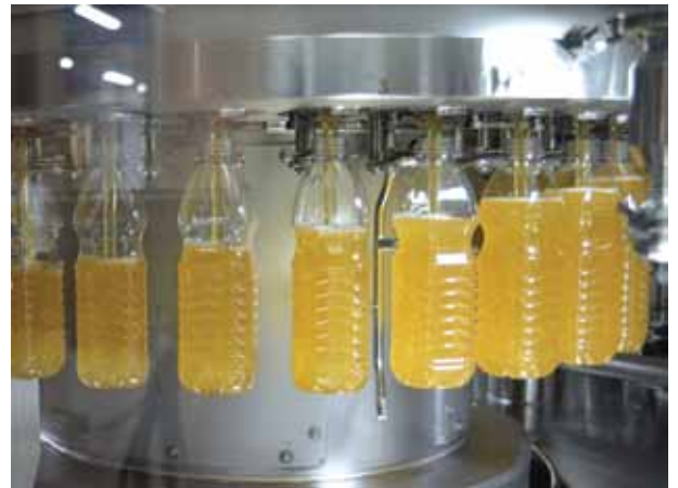
Combi Predis™/Capdis™ FMa is based on the dry-preform and cap decontamination technology
